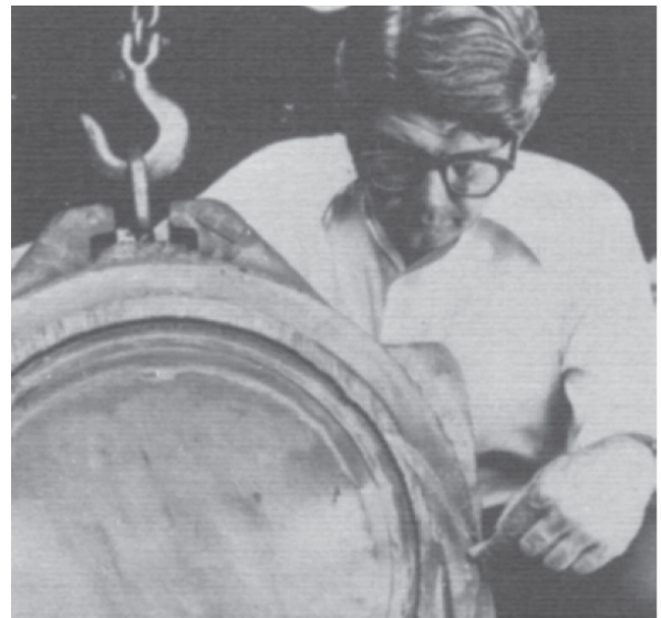
20 inch valve with NITRONIC 60 weld overlay on the seat and disk, operating in 400 °C (750 °F) conditions, lasting 140 days without galling.
